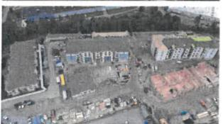
Currently under construction, this multi-family apartment complex is comprised of 168 units across 4 buildings. 2 of the 4 wood framed buildings are constructed on a concrete podium which provides underground parking. The complex also includes 4 separate outdoor garages, a community clubhouse, pool, dog park, running trail and additional outdoor amenities. Stateside worked closely with the developer and architect to optimize the design within the project's set budget parameters.
